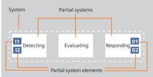
To attain a safety integrity level, the respective certification of the individual components is no longer sufficient. Now, the complete safety function must meet the defined requirements. This is why these standards call for an accurate calculation of the failure rates for all relevant electromechanical components.
