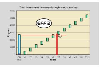
Comparison of Siemens make Eff1 and Eff2 motors with any other make having efficiency same as Eff2 specified in IS:12615-2004
