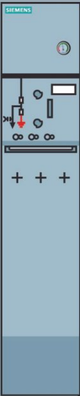
Typical Ring Main Feeder -R- :- 630A
